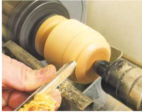
▲ Pic.4 He starts shaping the apple with the spindle gouge, with the top at the tailstock end. Keep the flute pointing in the direction of the cut and the handle tucked into your side
